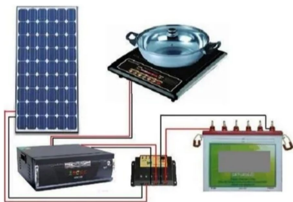
Fig. 8 Solar electric cooking system (Indiamart, 2024)
